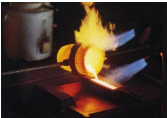
Guss eines Standardgoldbarrens (Foto: Argor-Heraeus SA)
